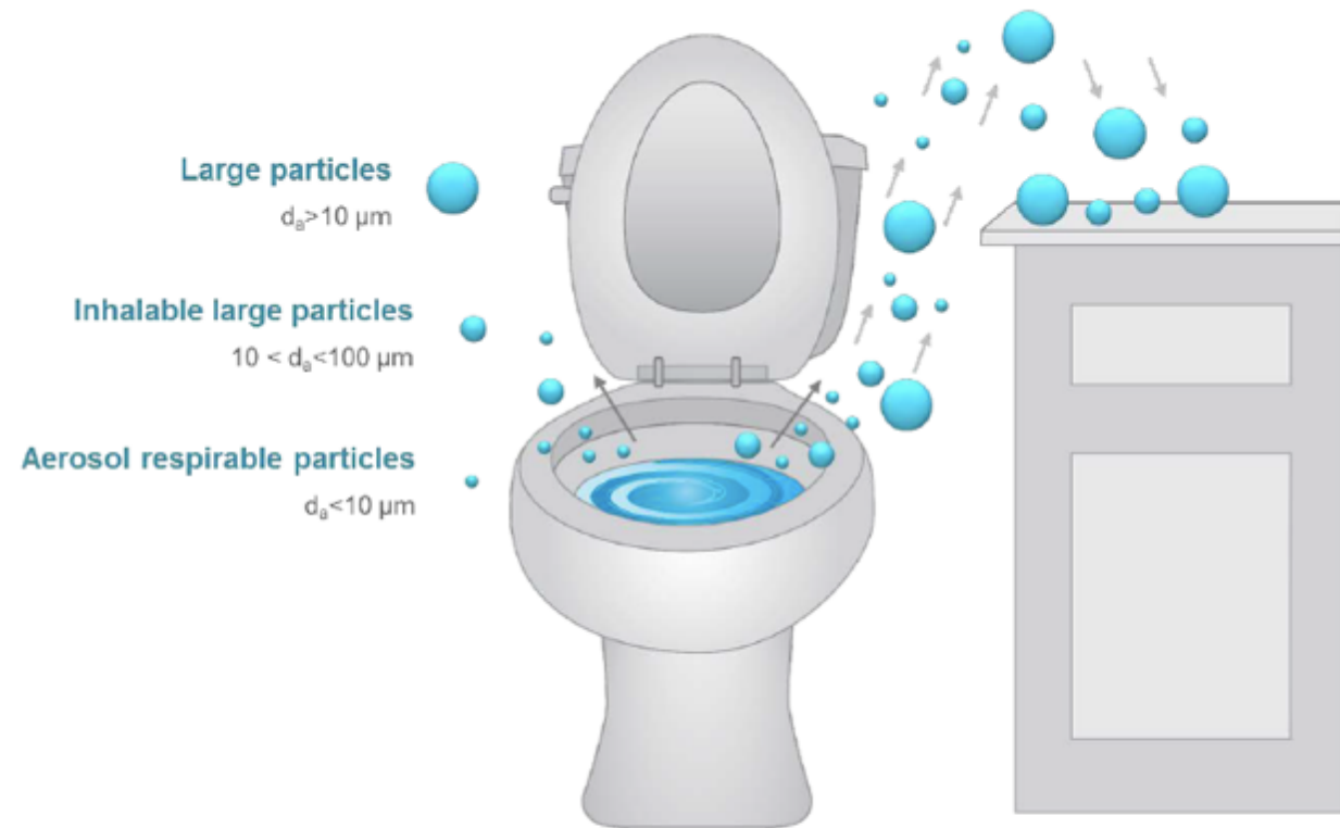
Figure 4-2. Toilet flush showing aerosol and particle deposition.
