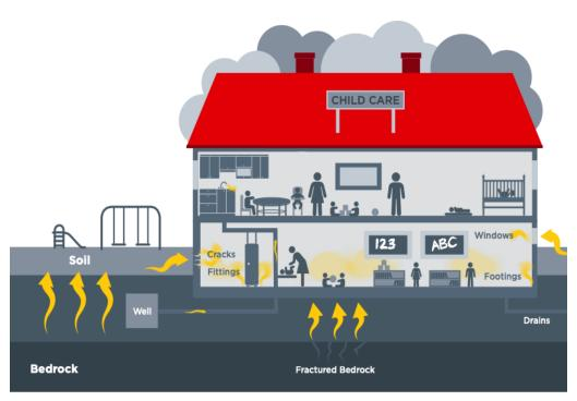
Radon is a radioactive gas that is the leading cause of lung cancer in non-smokers. It is released when uranium breaks down in the ground, and can enter child care settings in the various ways pictured here. Mitigation strategies can reduce this exposure in both new and existing structures.
